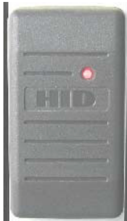
Figure 2-15 Bi-color LED in a Security Device
